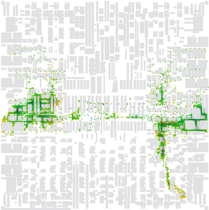
Fig. 10 Gigahertz clock net for the chip U3
