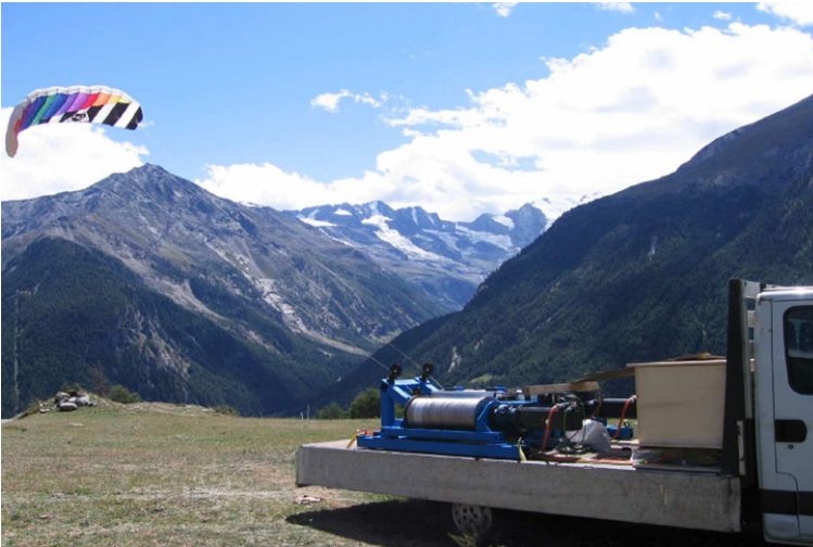
Fig. 8 Automatically controlled kite for energy production [12]
